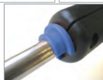
Orifice Indicator located on lance
